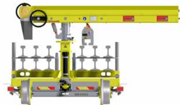
Loading diagram with 12 rails max. on 2 levels
