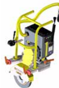
BLDC electric motor E³ grinding disc module
