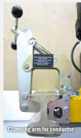
Clamping device for grooved rail
