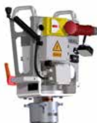
Electric motor cup wheel module
