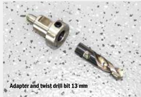
Drill bit, adapter and coolant ejector pin
