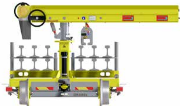
Loading diagram with 12 rails max. on 2 levels
