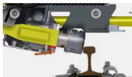
Maximum swivelling range 32° external and 80° internal
