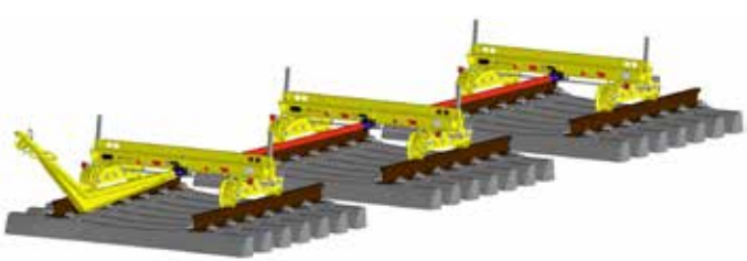
ROLLY 52.16 Version 5 with pivot plate, parking brake and uprights - 8269900040 Drawbar - 4511850180 Connecting rods - 8820032000
