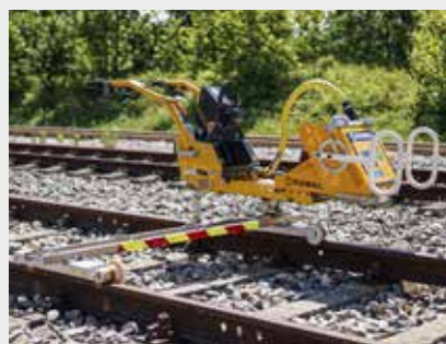
ROWRENCH 30.76 E³ Electric Precision Power Wrench
