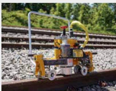
ROGRIND 13.45MD E³ Welding Joint Grinding Machine
