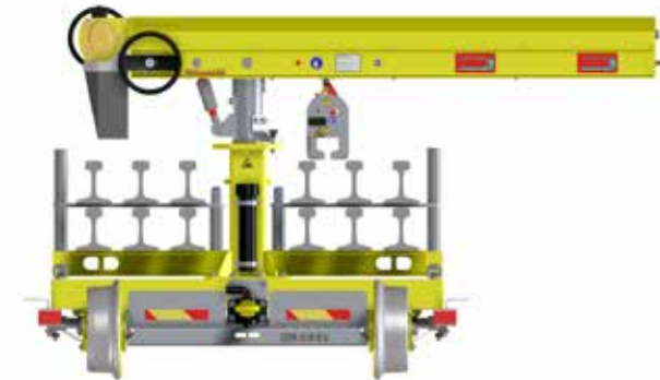
Loading diagram with 12 rails max. on 2 levels
