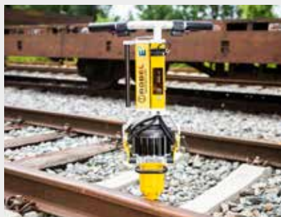
ROMPACT 30.20 E 3 Battery Powered Impact Wrench
