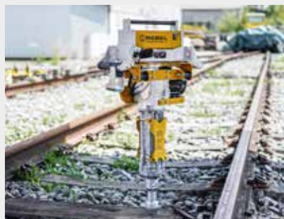
ROSPIKE 33.25 E 3 Battery Powered Spike Driver
