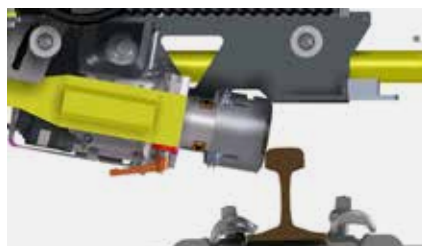
Maximum swivelling range 32° external and 80° internal
