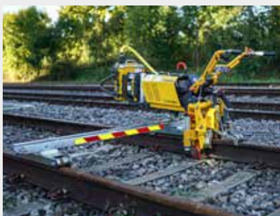
ROCLIP 34.01 E³ Akku-Clipmaschine
