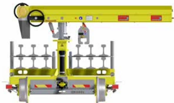
Loading diagram with 12 rails max. on 2 levels
