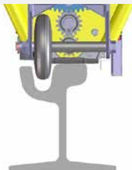
Conversion kit for grooved rails – outrigger, guide roller and copying roller – 8489910003
