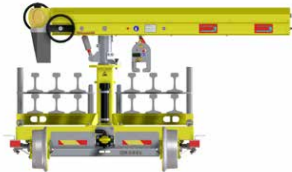
Loading diagram with 12 rails max. on 2 levels
