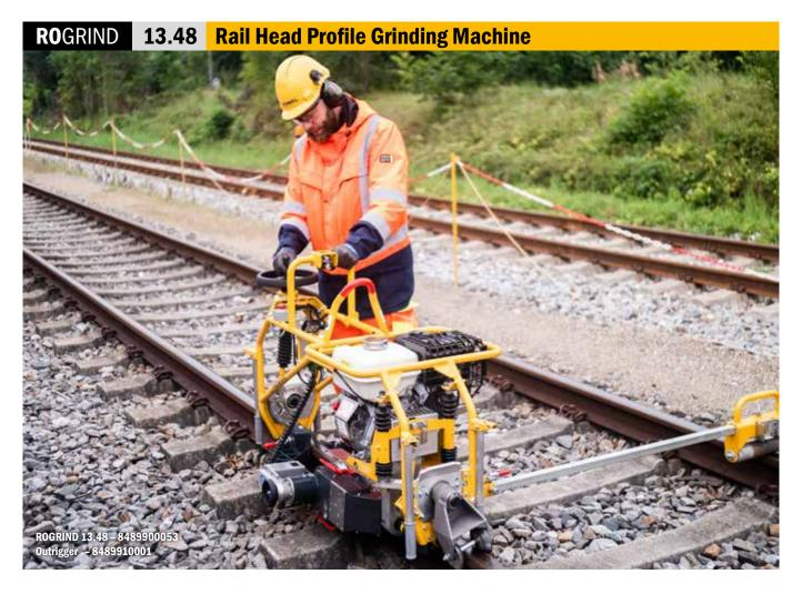
For true-to-form grinding of the rail head after welding work to restore a perfect profile.
