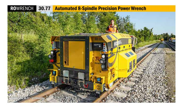
For simultaneous tightening or loosening of up to 8 rail fastenings in one step.
