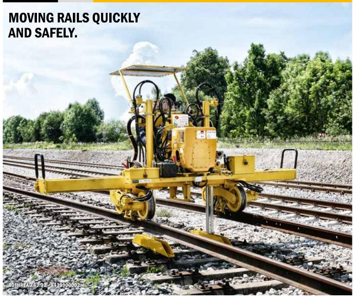
For continuous gradual repositioning of rails to the desired track gauge.
