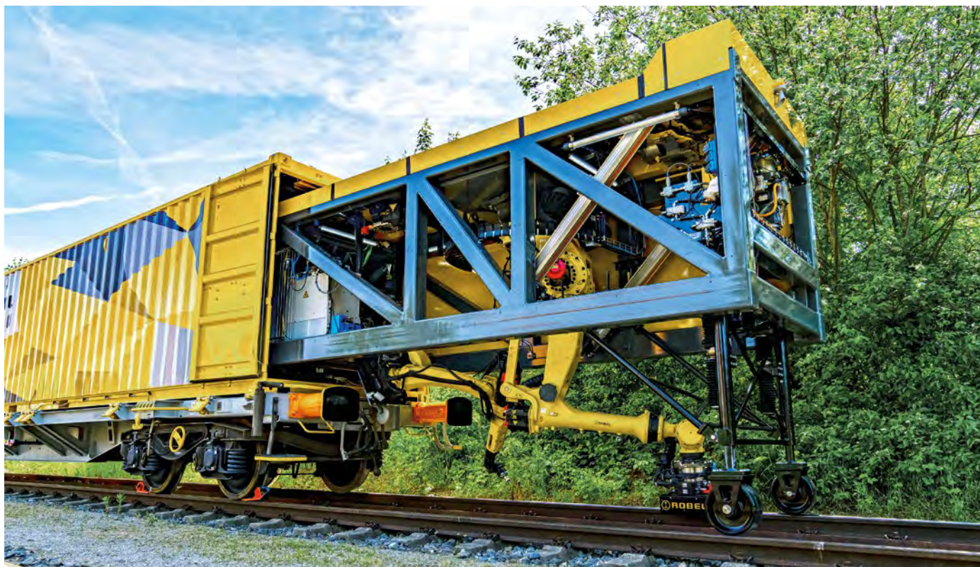
Fig. 2: The prototype for a maintenance container with fully automated robots was presented at iaf 2022.
