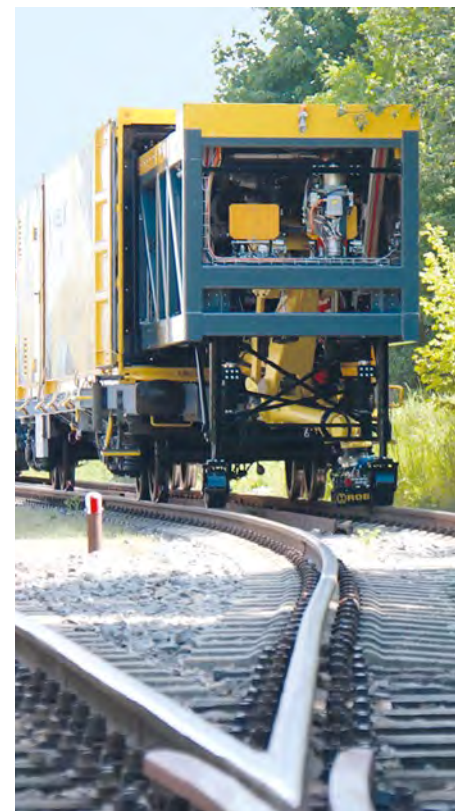
Fig. 1: Turnout maintenance is one of the first areas of application for automation on tracks.
