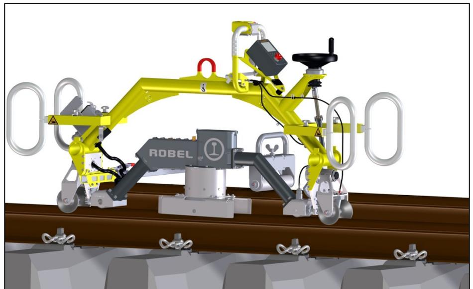
**Fig. 5:** Safety in every position: the deadman's brake on the side guide rollers is particularly effective for side grinding and on level ground.
