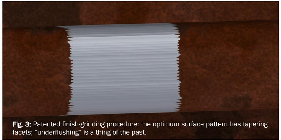
Fig. 3: Patented finish-grinding procedure: the optimum surface pattern has tapering facets; “underflushing” is a thing of the past.
