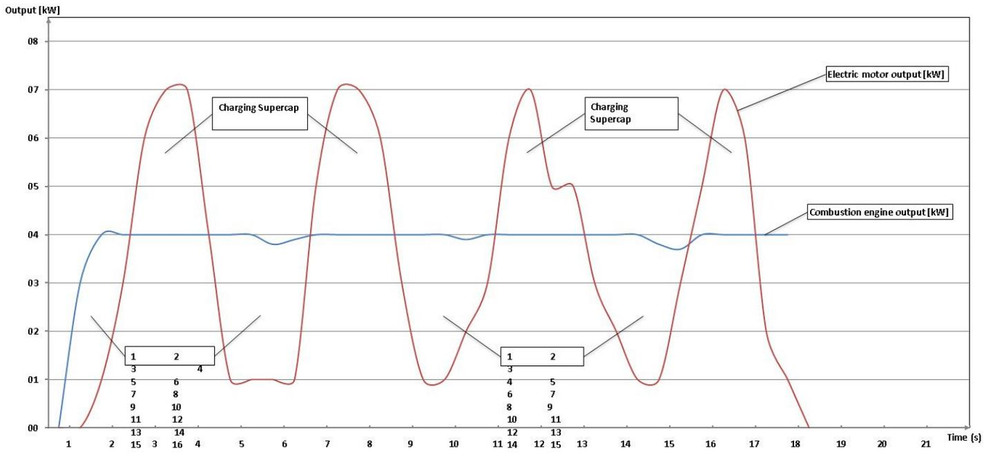
**Fig. 4:** Additional energy due to Supercaps: power curve of internal combustion engines and electric motors during grinding of a weld joint thing of the past
