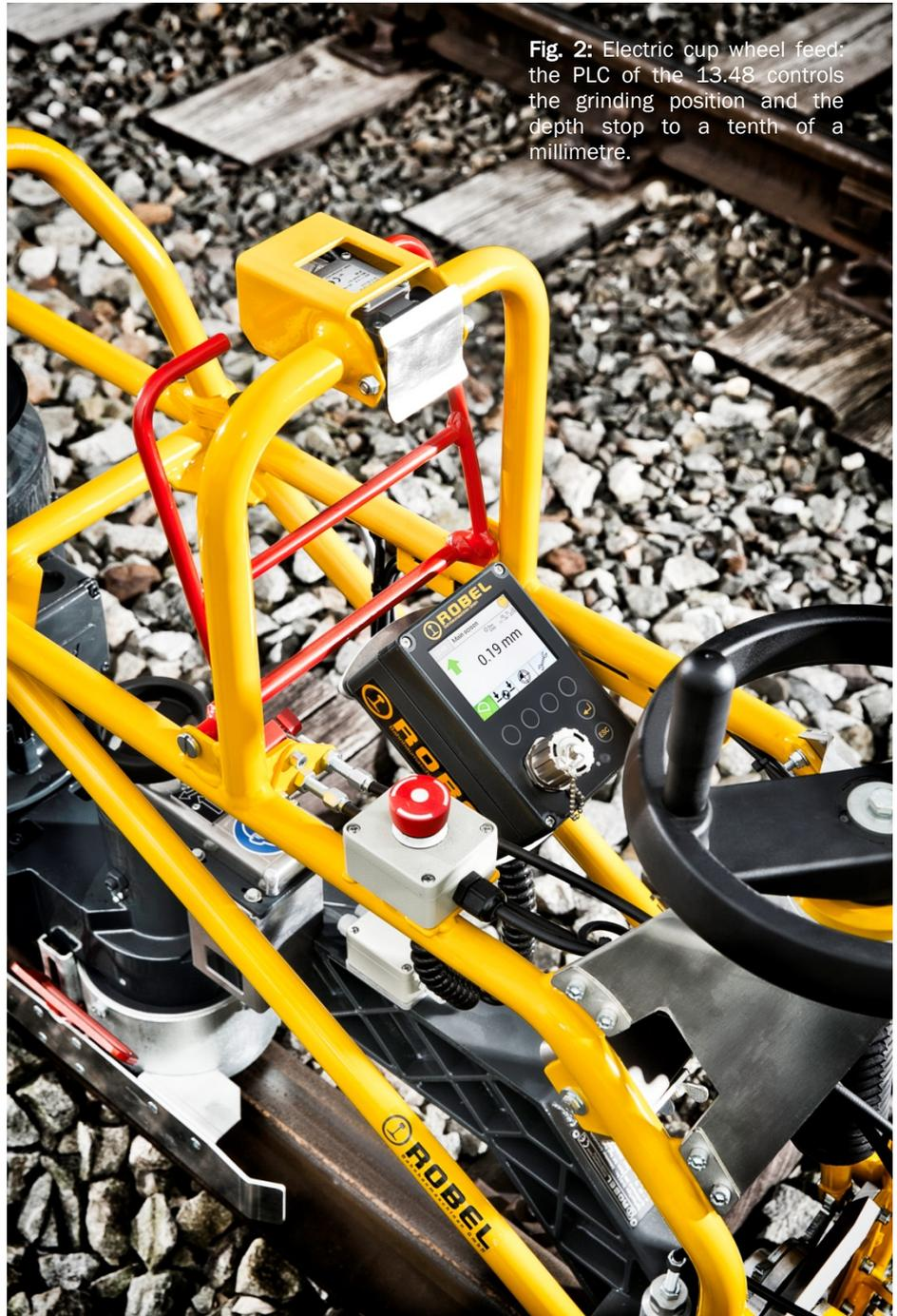
Fig. 2: Electric cup wheel feed: the PLC of the 13.48 controls the grinding position and the depth stop to a tenth of a millimetre.
