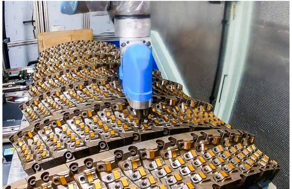
Fig. 9: Robot support while replacing the cutter inserts on the Romill rail milling machine
