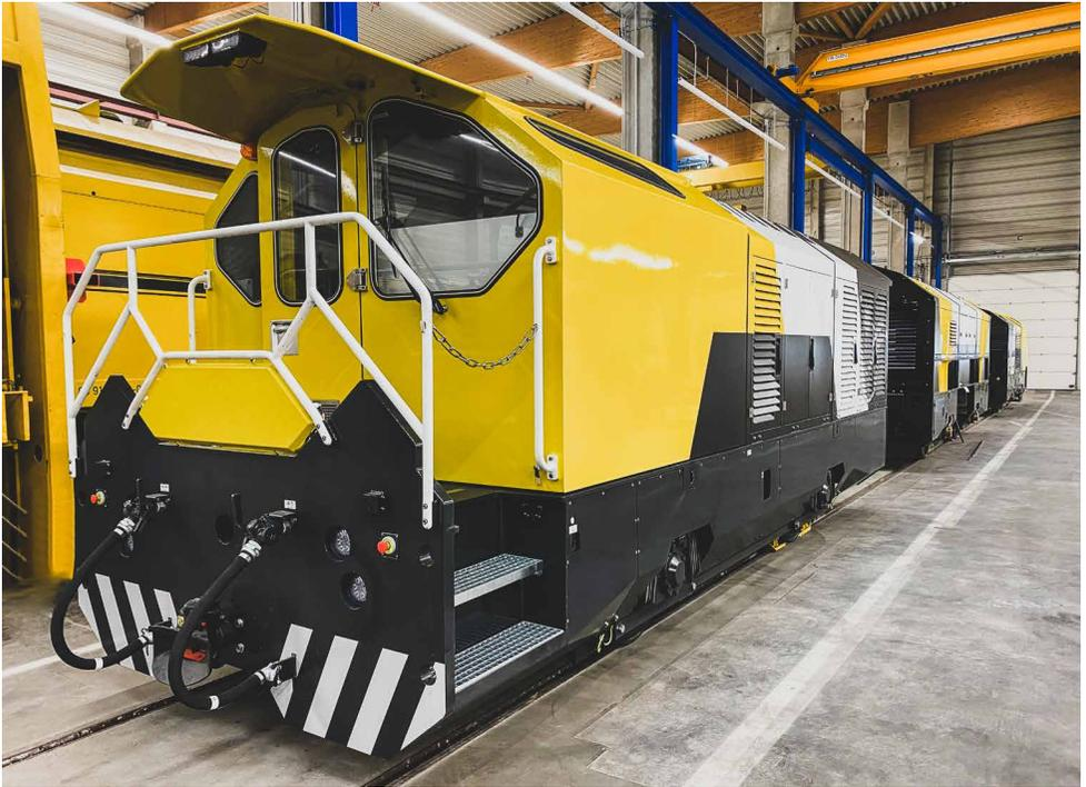
Fig. 11: Romill CMS3 rail milling train with hybrid drive during manufacture
