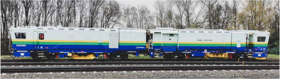
Fig. 8: Robel rail milling train for Japan with milling, polishing and measuring units
