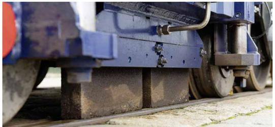
Fig. 6: Rubbing stone technology to generate a rail surface optimised for noise
