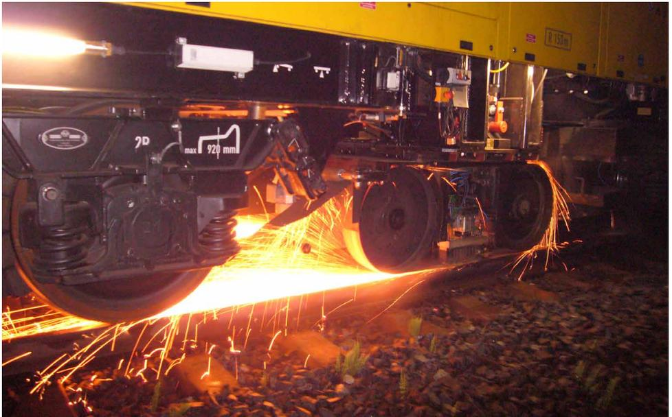
Fig. 5: Belt grinder for finishing after rail milling
