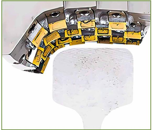
**Fig. 7:** Rail milling technology: precise reprofiling of the rail due to the shape of the milling cutter
