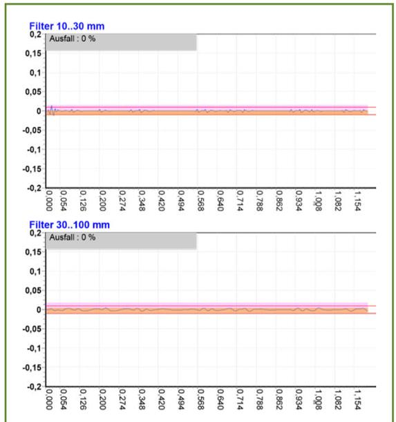
Fig. 10: Resulting surface with the lowest roughness after finishing with oscillating rubbing stones
