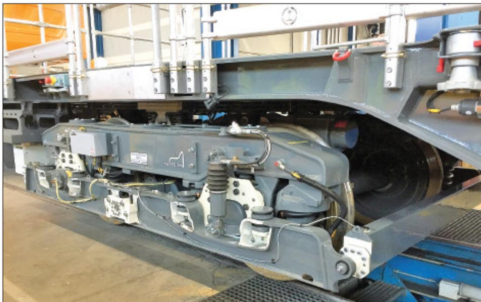
Left: Frame mounted on the bogie to house ultrasonic and eddy current test equipment.
