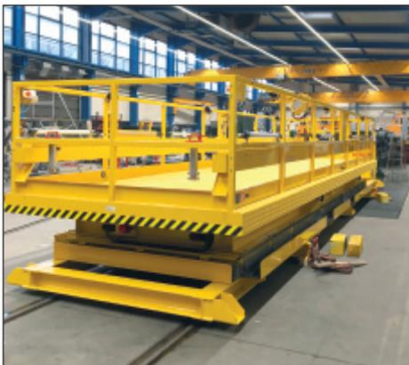
**Above left: Scissor lift mounted on its ISO twistlock frame.**
