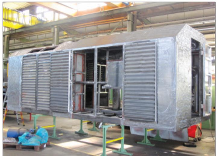
Power Car A - the driver's cab welded and ready for painting (above left) and the pre-assembled engine room (above right).
