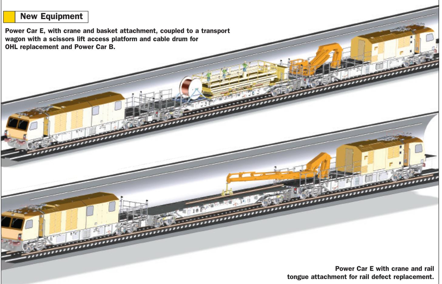
Power Car E with crane and rail tongue attachment for rail defect replacement.
