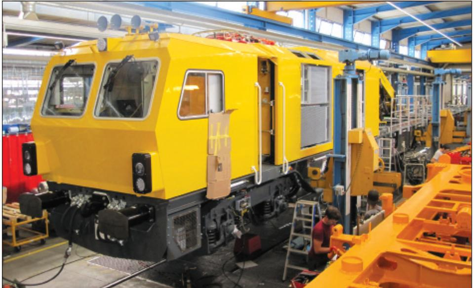
Power Car E - viewed from the front (above) showing the completion of painting, assembly of all major component including bogies, engine and transmission system and final assembly of hydraulic, electric and pneumatic systems. The crane installation at the rear (below).
