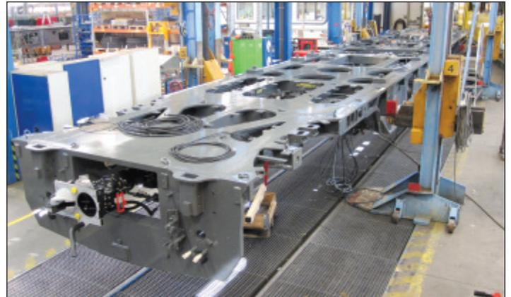
**Power Car B (No: 1) - the painted subframe with the coupling installed and part installation of hydraulic, electric and pneumatic systems (above).**
