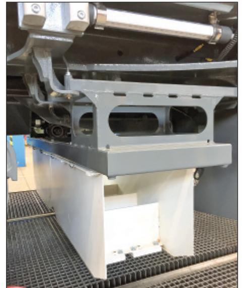
Bracket for geometry and rail profile equipment (above left) and bracket for visual recognition equipment (above right). The white boxes simulate equipment for the ride tests.
