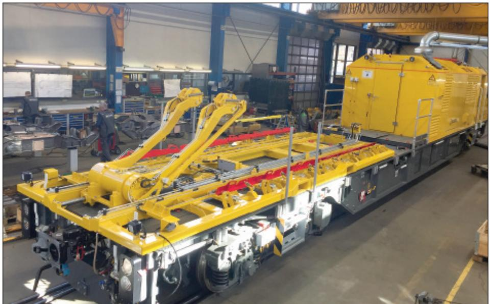
**Above right: On-off loading device with armature mounted on hydraulic rotary actuator mounted on Power Car A.**
