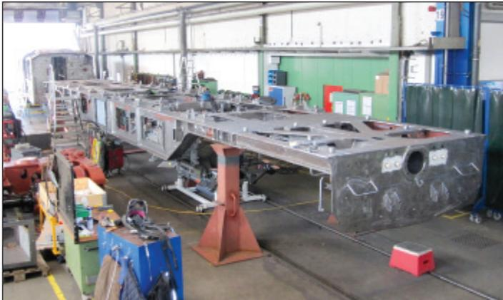
**Power Car B (No: 2) - the subframe complete with part assembly of hydraulic, electric and pneumatic systems, prior to strip down and painting (above).**
