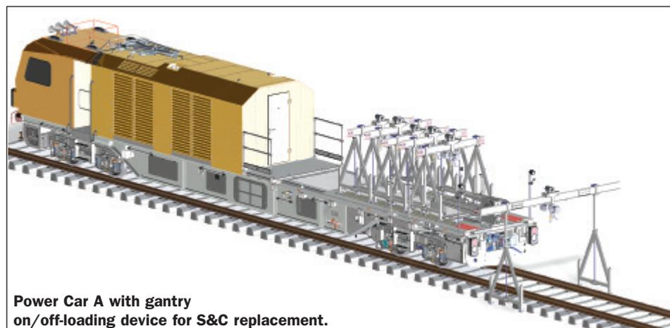
Power Car A with gantry on/off-loading device for S&C replacement.
