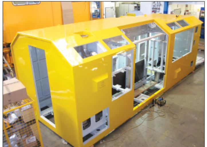
**Power Car B (No: 1) - the painted cab and start of final assembly (above left) and welfare module painted and start of final assembly (above right).**
