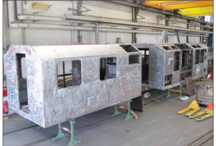
**Power Car B (No: 2) - the driver's cab after painting (above left) and the engine room and welfare module frame before painting (above right).**
