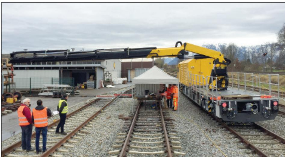
**Above: Testing the crane on Power Car E at Robel's workshops at Freilassing.**
