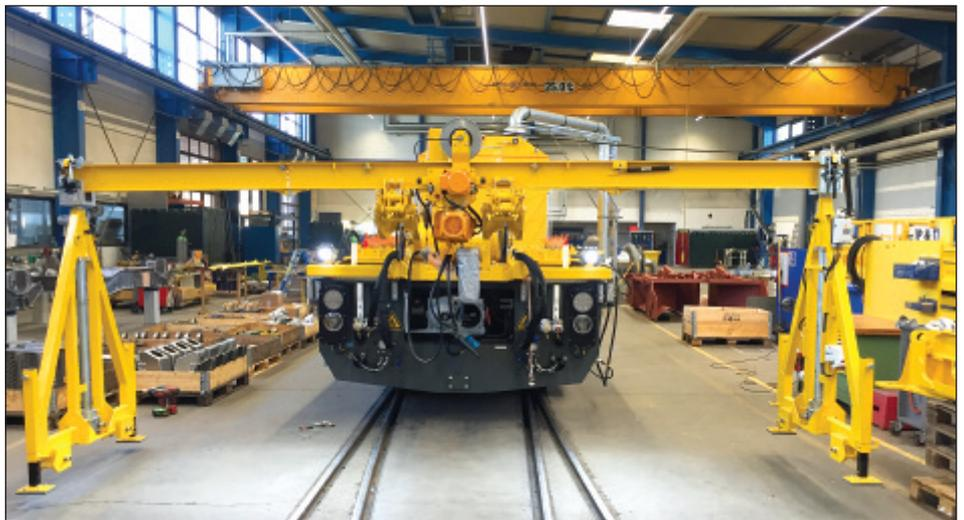
**Above: Gantry on-off loading device with crossbeam and legs deployed.**
