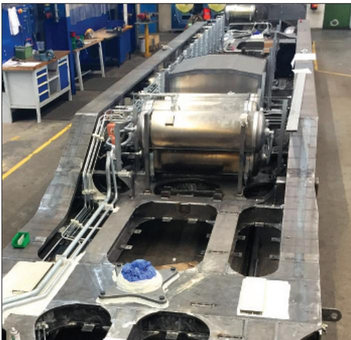
Above: Power Car B's sub-frame with the pneumatic system fitted.
