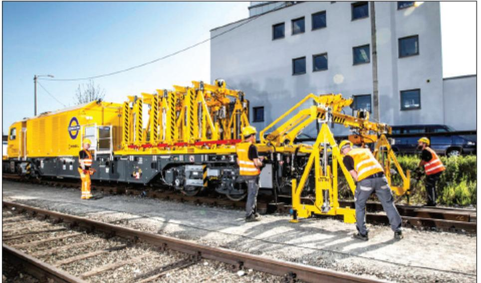
Above: On/off-loading module mounted on Power Car A off-loading one of six electrical gantries. Part of Case Study 1 to change F switches within a tunnel.
