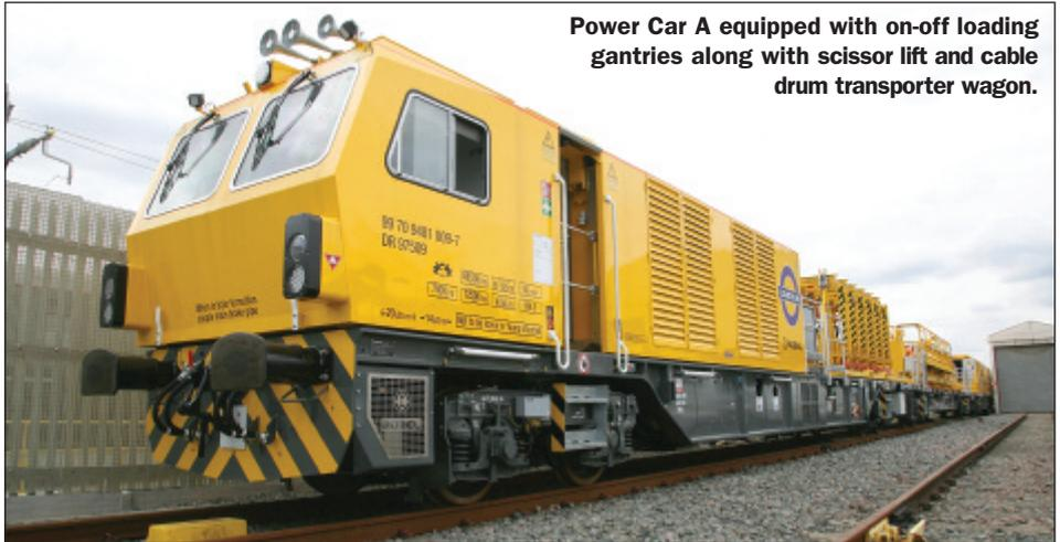
Power Car A equipped with on-off loading gantries along with scissor lift and cable drum transporter wagon.
