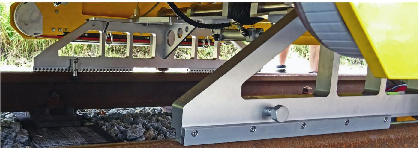
**Image 9:** The sensor head of the RMF 1100 measuring system captures the longitudinal corrugations of the rail after grinding.
