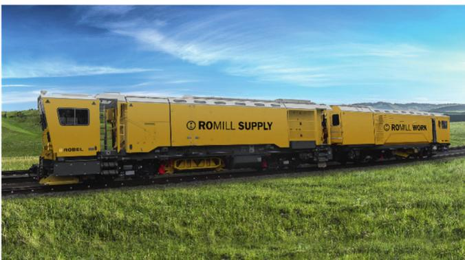
**Image 1:** The two-part ROMILL rail milling system is Robel's first product for reprofiling rails.
