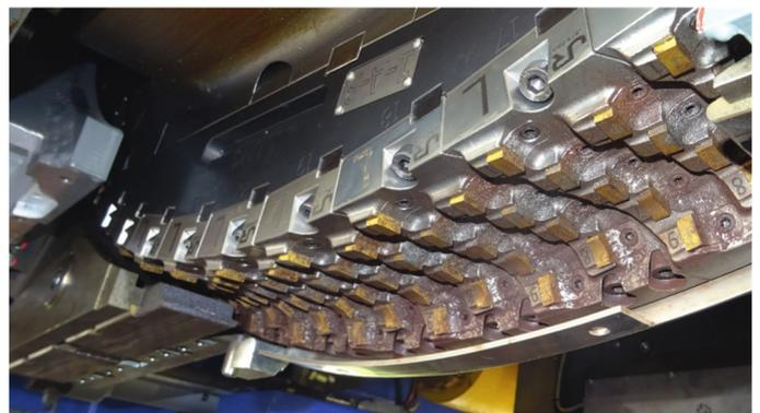
**Image 2:** The cutting inserts positioned vertically on the milling wheel allow for an increased number of cuts for even more effective milling.
