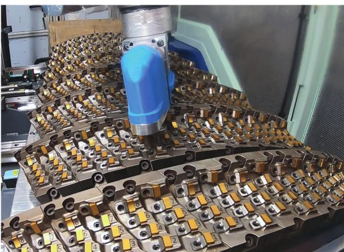
**Image 5:** A collaborating robot tightens and loosens the cutting inserts.
