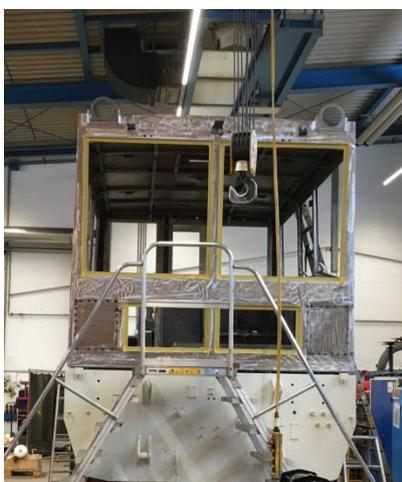
Fig. 11: A complete refurbishment or replacement of the cabin allows for the installation of additional windows with modern fixing methods.
