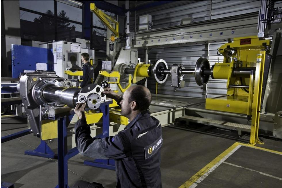
Fig. 8: Double-cylinder axle press for automatic press-fitting and removal of wheels and brake discs with digital monitoring and recording
