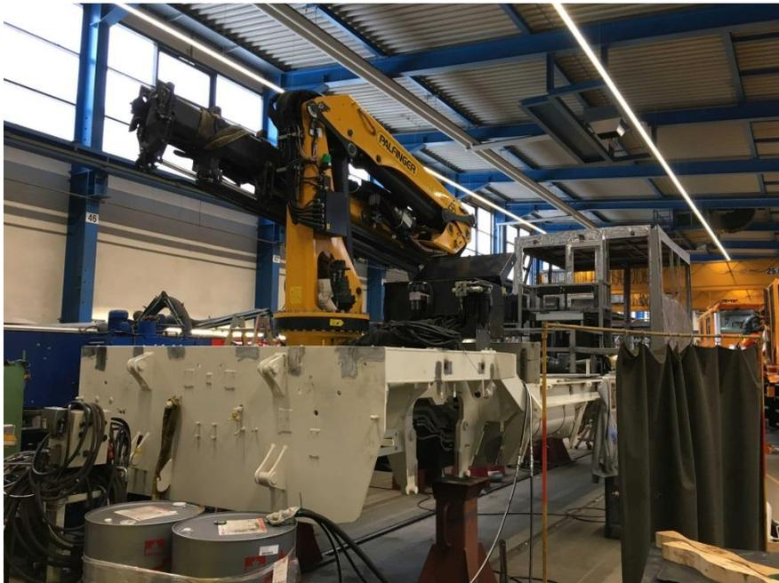
Fig. 14: Manufacturer know-how flows into the assembly processes of a retrofit; here the body shell before painting.
