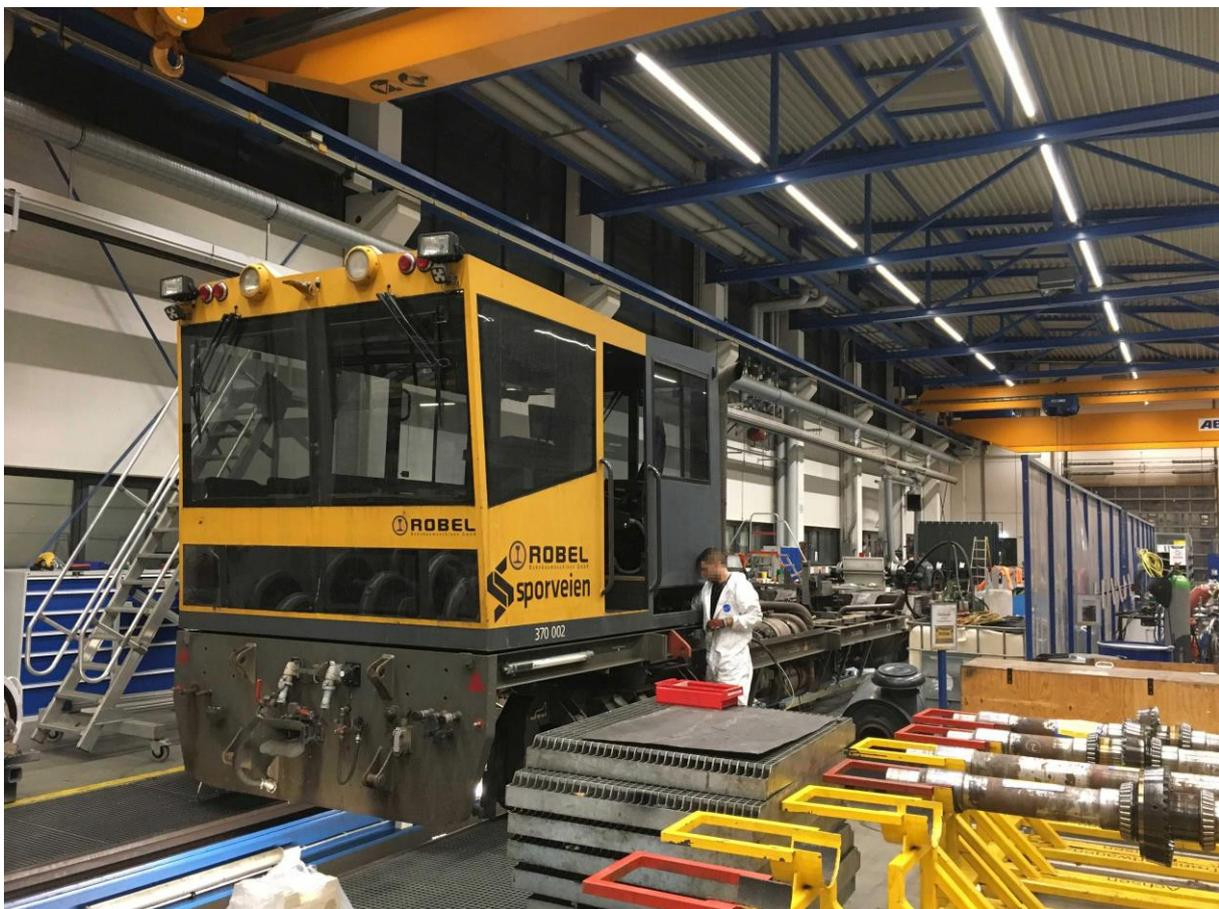
Fig. 3: After the initial investigation the track vehicle is fully dismantled
