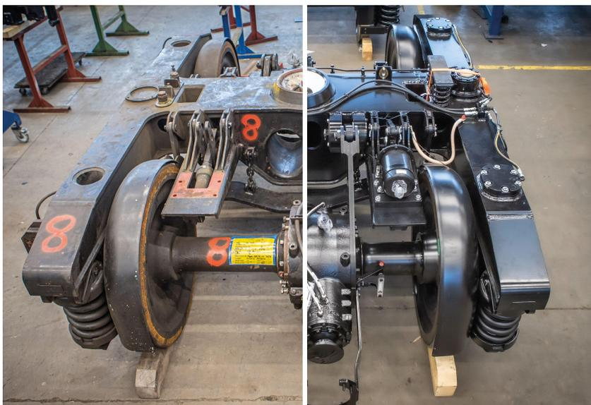
Fig. 1: Bogie of a 09-3X tamping machine before and after overhaul Source of all Figures: Robel
