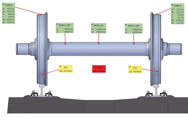
Fig. 5: The test record of the laser measuring instrument shows whether wheelset, wheel disk and brake disk are within the wear tolerances (=green), are close to the upper or lower limit (=yellow) or are outside the tolerance (=red).
