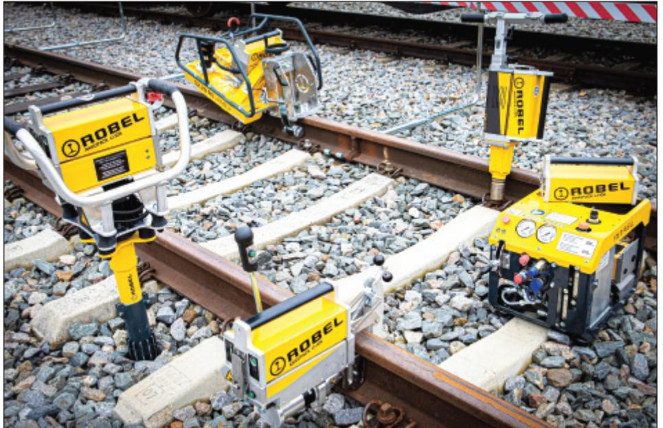
welding joint grinding machine and a hybrid railhead profile grinding machine - that can either be driven by a 2kWh battery, a 6kWh battery or a power supply.
