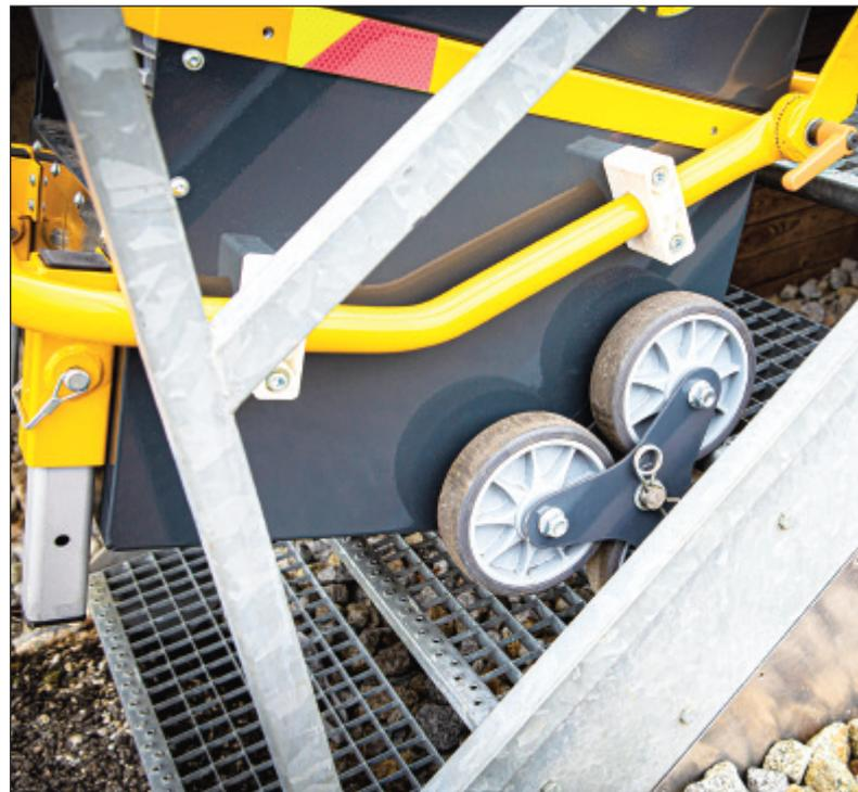
**Robel rail/road trolley has been specially designed for easy transport of the high capacity battery pack and other materials, which might be required at the worksite.**
