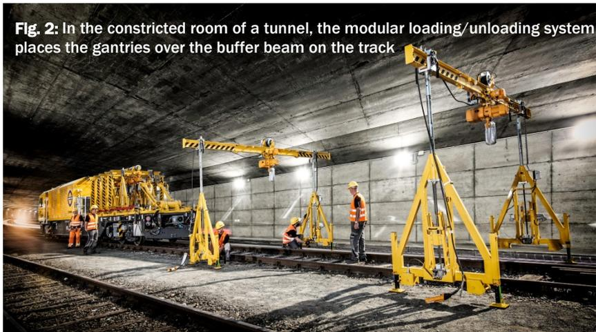
**Fig. 2:** In the constricted room of a tunnel, the modular loading/unloading system places the gantries over the buffer beam on the track
