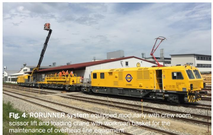
**Fig. 4:** RORUNNER system equipped modularly with crew room, scissor lift and loading crane with workman basket for the maintenance of overhead line equipment.
