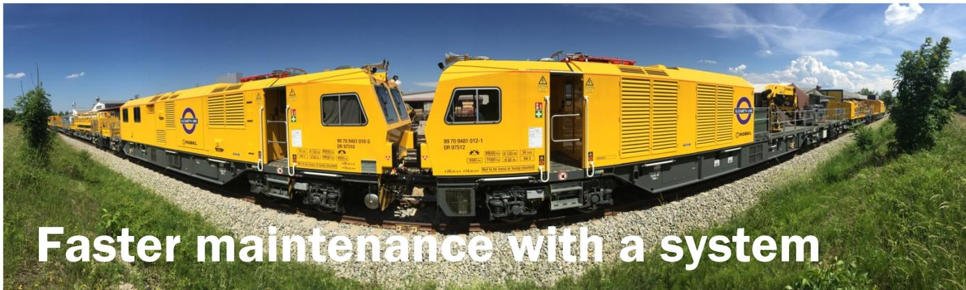
**Fig. 1:** RORUNNER system for the London Elizabeth Line consists of two train formations, each with two track vehicles and one transport transport wagon.
