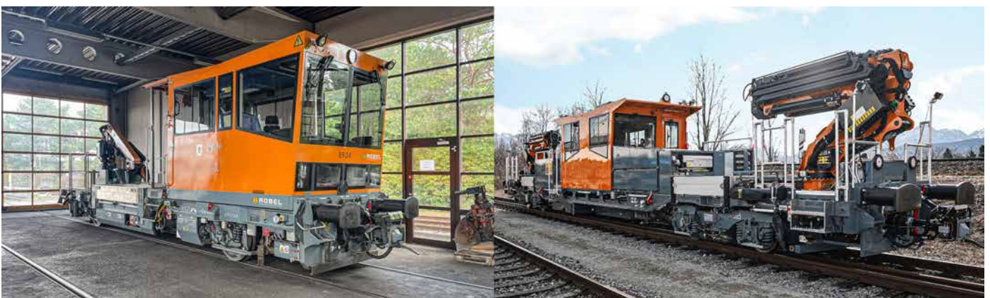
Fig. 3: From one to two cranes: the existing fleet of track maintenance vehicles will be supplemented by ten three-axle hybrid track maintenance vehicles as of 2024
