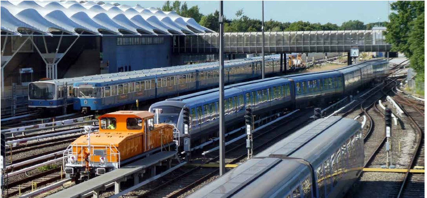
Fig. 2: To reduce CO 2 emissions, electric locomotives with additional battery equipment are used for traction tasks, among other things
