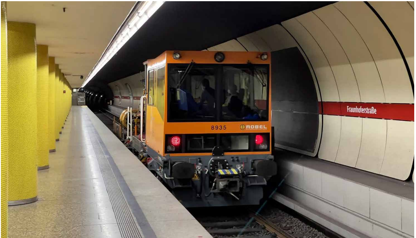
Fig. 1: MVG mainly uses heavy-duty small wagons for infrastructure maintenance on the underground
