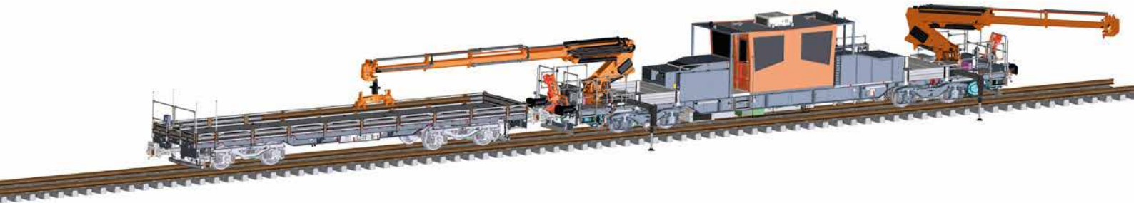
Fig. 4: As the Munich underground network does not have any facilities for turning, all units are designed for bi-directional working, with a crane on both vehicle ends and loading platforms at station level on both sides.
